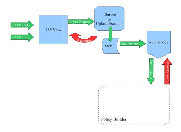
In the user interface of the Policy builder ,jsp dispatches the input stream of SOAP data asynchronously into Servlet Dispatcher (Upload Executor) which inturn uses a stub generated (using the Service WSDL) to invoke the web Service. Web Service interacts with the Policy Builder System and provides the derived output to the servlet. Sevlet will inform the jsp of the response through a the Ajax CallBack.
