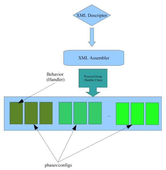
An External Descriptor file(builder.xml) is used to build the handler chain. This is kind of similar to Chain of Responsibility configuration for a handler set (/set of Behaviors). However behavior set is grouped into configurations or phases where each seperate set can be operated seperately..Policy extraction will be done for each phase and a security policy instance will be derived for each individual phase.
