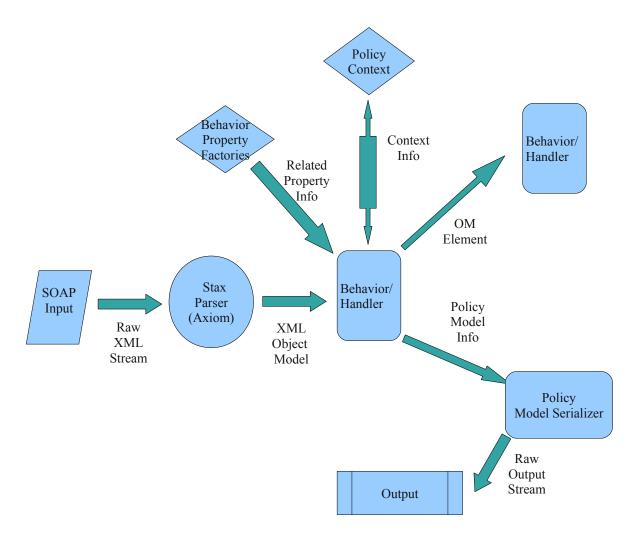
Axiom Object model and Rampart Security Policy Model is extensively used in the Policy Builder System.Policy Builder uses StaxParser (A Pull parser used in Apache Axiom) to generate XML Object Model and provide it as input to the handlers. Using the property information and other context information, underline security policy information is derived and inturn provided for Policy Model which is then made responsible for policy serialization.
