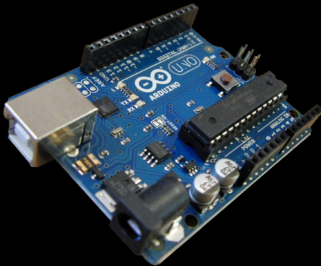
Arduino Uno board 8 bit Atmel AVR
