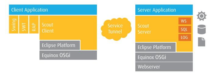
Illustration of a typical Scout application architecture:
