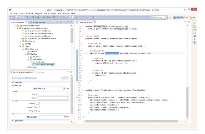
This screenshot of the Scout SDK shows how a dialogue form is created: The specifications of the MessageField highlighted in the Scout Explorer are listed in detail in the Scout Object Properties view and shown as Java code in the column to the right.
