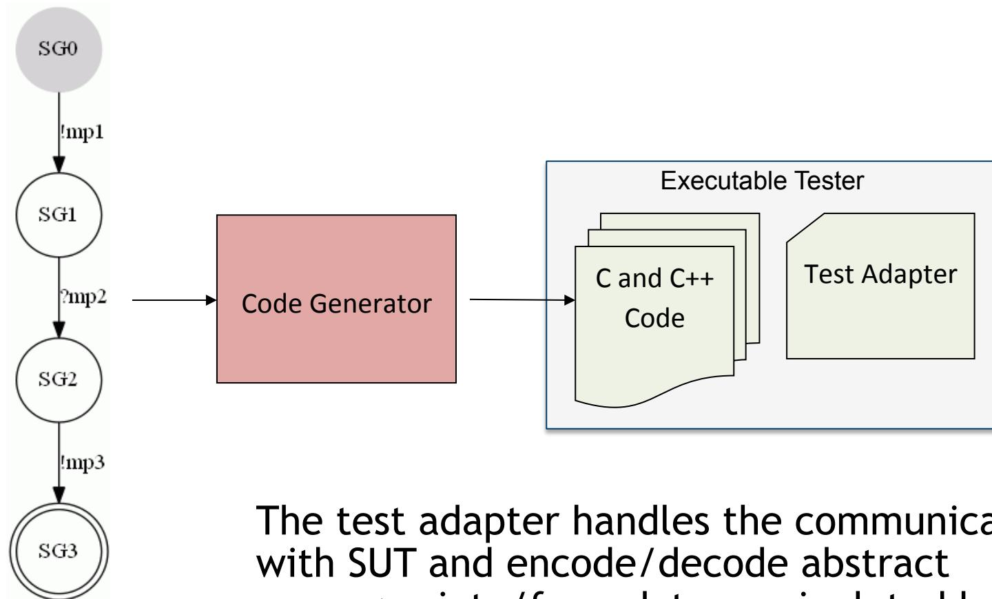
The test adapter handles the communication with SUT and encode/decode abstract messages into/from data manipulated by the SUT
