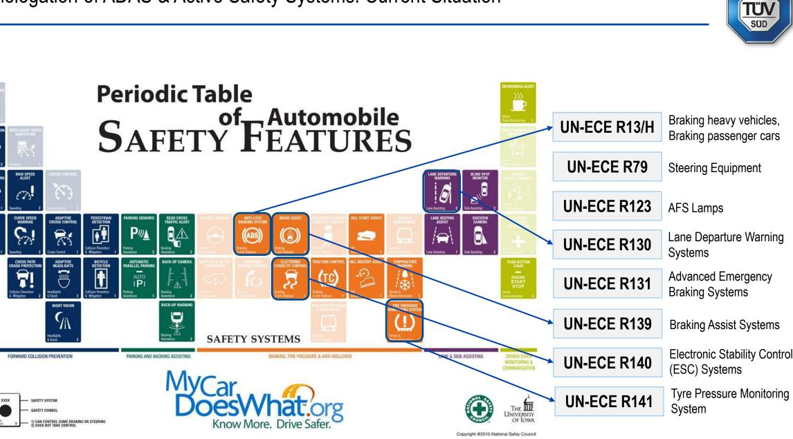
ECE-R 140 allows for simulation methods to support the homologation of electronic stability control systems (ESC)
