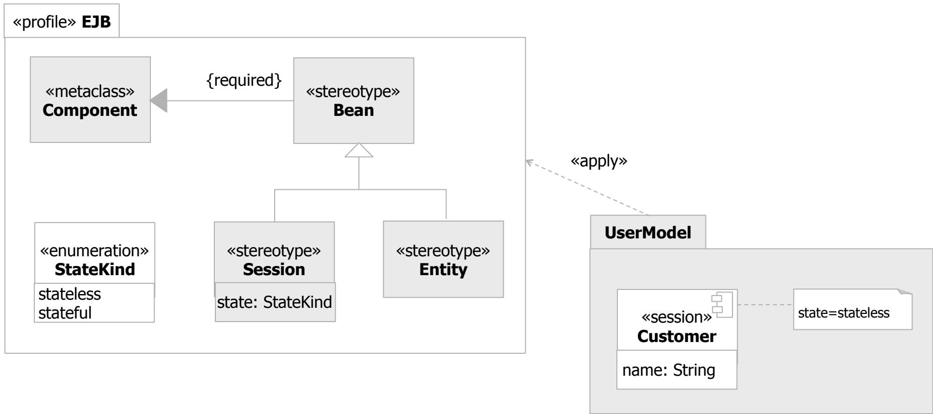
Applying a profile makes the profile extension available to the model packages to which it is applied.
