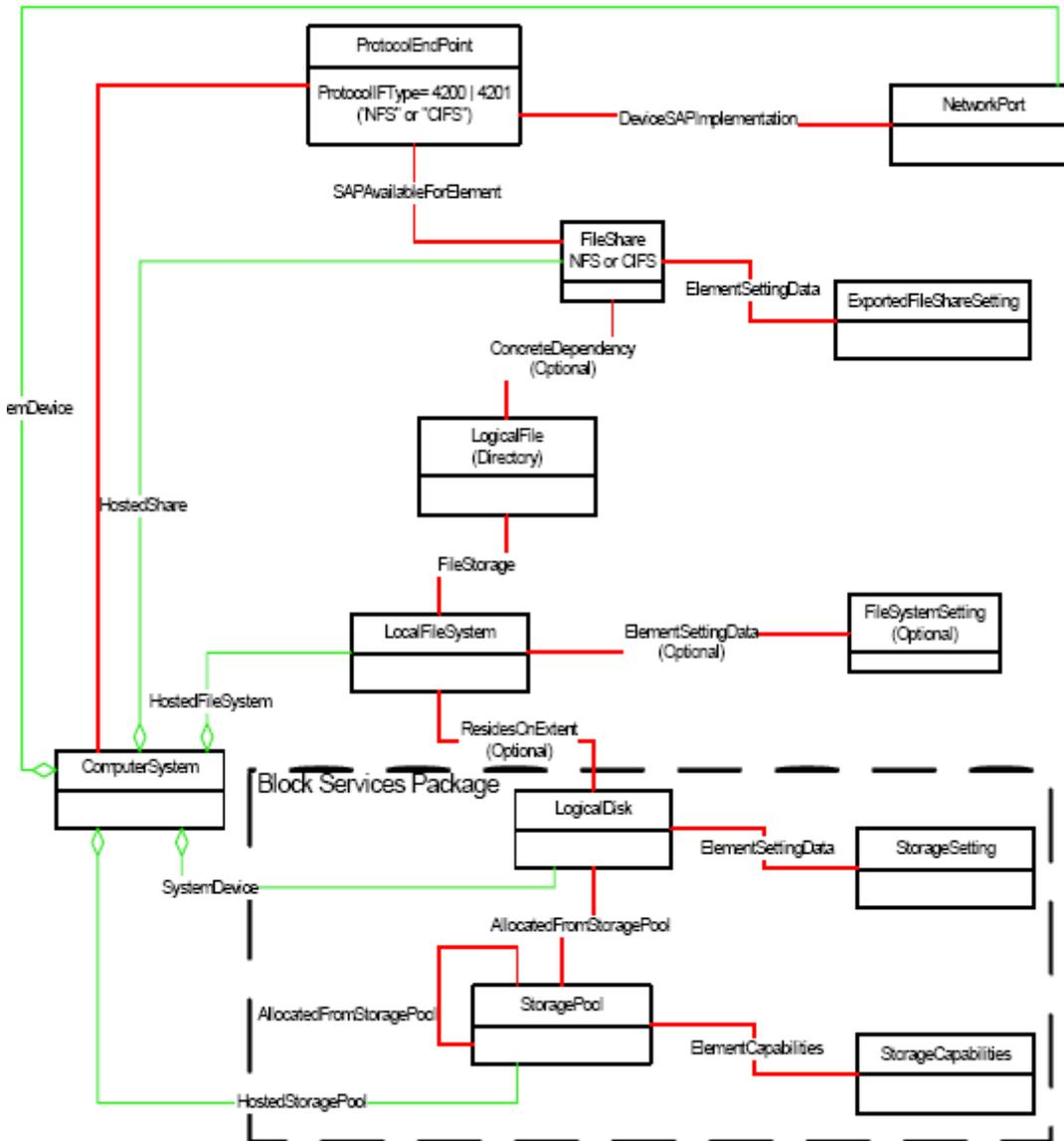
As with Arrays, the “top level” ComputerSystem of the Self-Contained NAS typically isn’t a real ComputerSystem. It is merely the ManagedElement upon which all aspects of the NAS offering are scoped.
