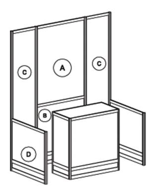
Dimensions listed for the panels are the true measurements for each panel shown. If you plan to overlay your graphics on the existing panels, you will need to <u>subtract ¼"</u> from each measurement listed.
