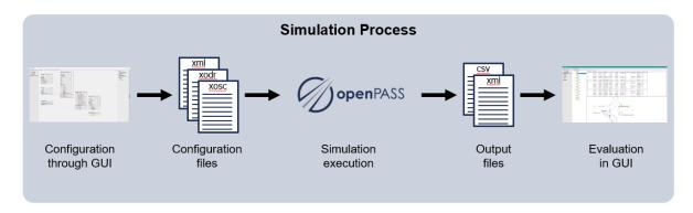
The illustration above shows the simulation process in openPASS. Over configurations in the GUI the user set up the desired simulation run. Basically, the GUI supports the user to set up the simulation in accessing and writing .xml, openSCENARIO and openDRIVE files. After the setup of the configuration files the simulation can be executed. As an output .csv and .xml files are generated. For the future, the evaluation over the GUI should be available which is yet still under development.
