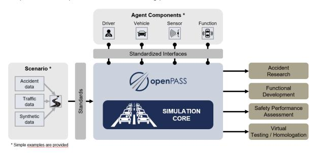
The platform is built up in a modular manner. The simulation core calculates different simulation runs. Scenarios and agent components can connect to the core over standardized interfaces like OpenSCENARIO, OpenDRIVE, OSI and FMI. The openPASS WG provides
